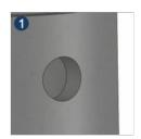
The hole has to be drilled according to the tolerance  $\pm 2$
