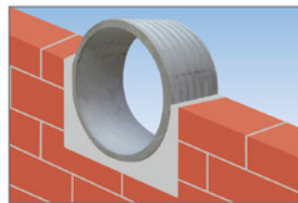
Fitting in brickwork
