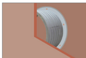
Fix wall sleeve in casing with casing supports
