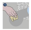
Clean casing pipe/core drilling and carrier pipe. Carrier pipes must be suitable, dimensionally stable and without damage in the sealing area. Core drillings have to be made true to scale and with a smooth inner side.
